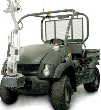
A Kawasaki Mule retrofitted with the Pronto4™ Strap-on Autonomy System and a retrofit manipulator arm.
