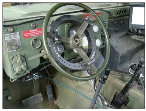
A Pronto4™ Strap-on Autonomy System Series 2 installed on a miltary HMMWV.
